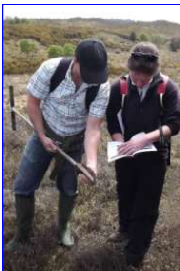
Soil auguring to ascertain the physical characteristics of the soil underlying the heathland at Agglestone.
